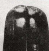
Other Make No. 2—Right hand point worn shorter than left. Tip extremely rough.
